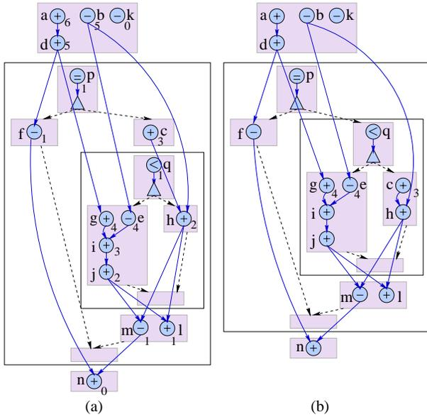
**Figure 2: Reverse Speculation for the waka benchmark (a) original design (b) after reverse speculation** has high priority since all the operations in its conditional branches depend on it.
