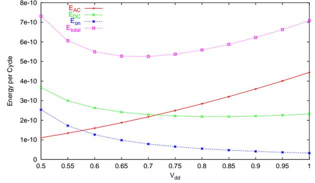
**Figure 2: Energy per Cycle for 70nm technology for the Crusoe processor:**  $E_{AC}$  is the switching energy,  $E_{DC}$  is the leakage energy and  $E_{on}$  is the intrinsic energy to keep the processor on.
