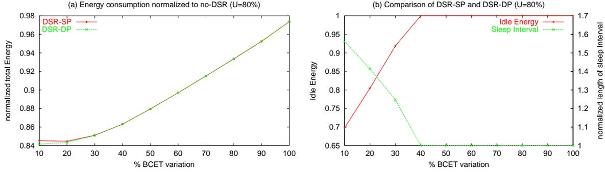
**Figure 2: Utilization,  $U=80\%$  (a) Comparison of total energy of DSR-SP and DSR-DP normalized to no-DSR (b) Comparison of average idle energy and average sleep interval of DSR-DP normalized to DSR-SP**
