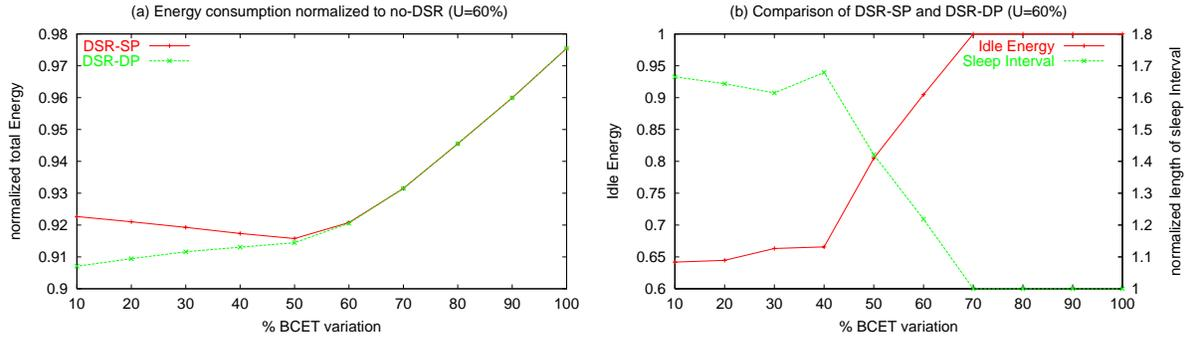
**Figure 3: Utilization,  $U=60\%$  (a) Comparison of total energy of DSR-SP and DSR-DP normalized to no-DSR (b) Comparison of average idle energy and average sleep interval of DSR-DP normalized to DSR-SP**
