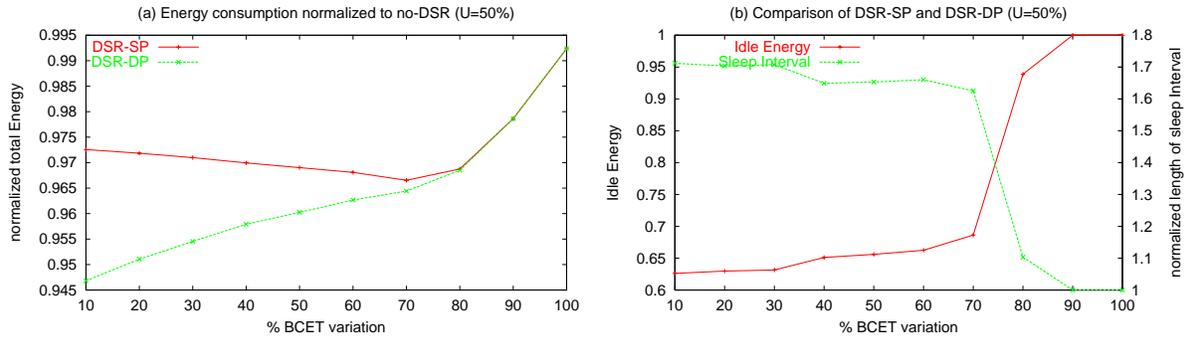
**Figure 4: Utilization,  $U=50\%$  (a) Comparison of total energy of DSR-SP and DSR-DP normalized to no-DSR (b) Comparison of average idle energy and average sleep interval of DSR-DP normalized to DSR-SP**
