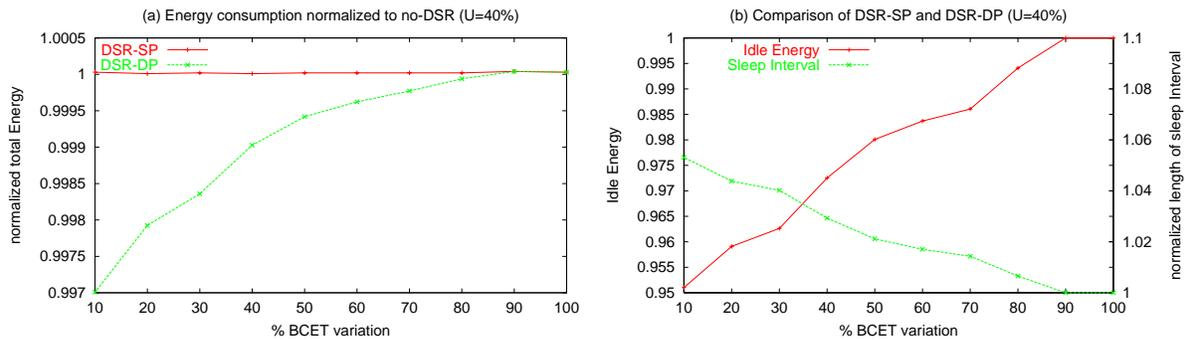
**Figure 5: Utilization,  $U=40\%$  (a) Comparison of total energy of DSR-SP and DSR-DP normalized to no-DSR (b) Comparison of average idle energy and average sleep interval of DSR-DP normalized to DSR-SP**
