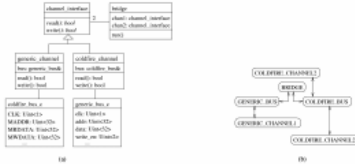
Figure 6 On Chip Bus Pattern: (a) Class Diagram (b) Object Diagram
