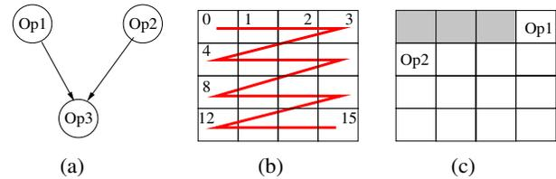
Figure 2. (a) *Sample DFG* (b) *Zig-zag topology traversal* (c) *Op<sub>3</sub> suffers a communication delay in this mapping*
