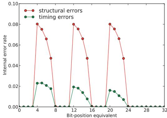
Fig. 10. Bit-level-equivalent error distribution in ISA (8,0,0,4) under 15% CPR.
