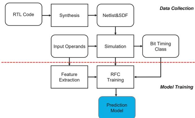
Fig. 3. Bit-level timing error prediction model construction flow.
