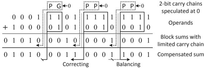
Fig. 2. Example of ISA addition arithmetic with 2-bit speculation, 1-bit correction and 1-bit error reduction. Faults only occur in the two right-hand paths. The 1<sup>st</sup> LSB of the central path can be corrected. The 1<sup>st</sup> LSB of the right path cannot be corrected, so the 1<sup>st</sup> MSB of the preceding sum is flipped.
