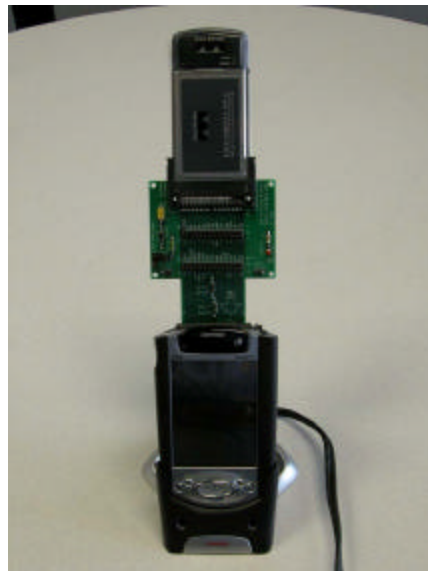
Figure 4. iPAQ fitted with the KAITEK PCMCIA Extender card for Power Measurements
