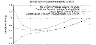
Figure 1: Energy consumption normalized to no-DVS
