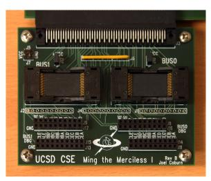
Figure 1: Our flash testing board The flash testing board can test two chips simultaneously and, combined with an FPGA board and a current meter, supports high-resolution timing and power measurements.
